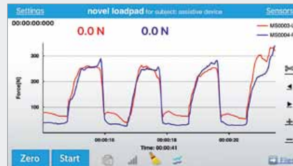
Forces on the handles of assistive devices (left and right)
